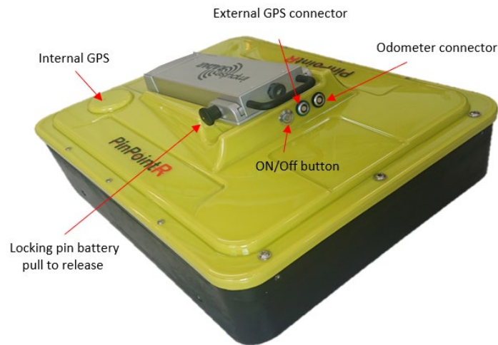
Figure 2 PinPointR antenna with a battery attached
